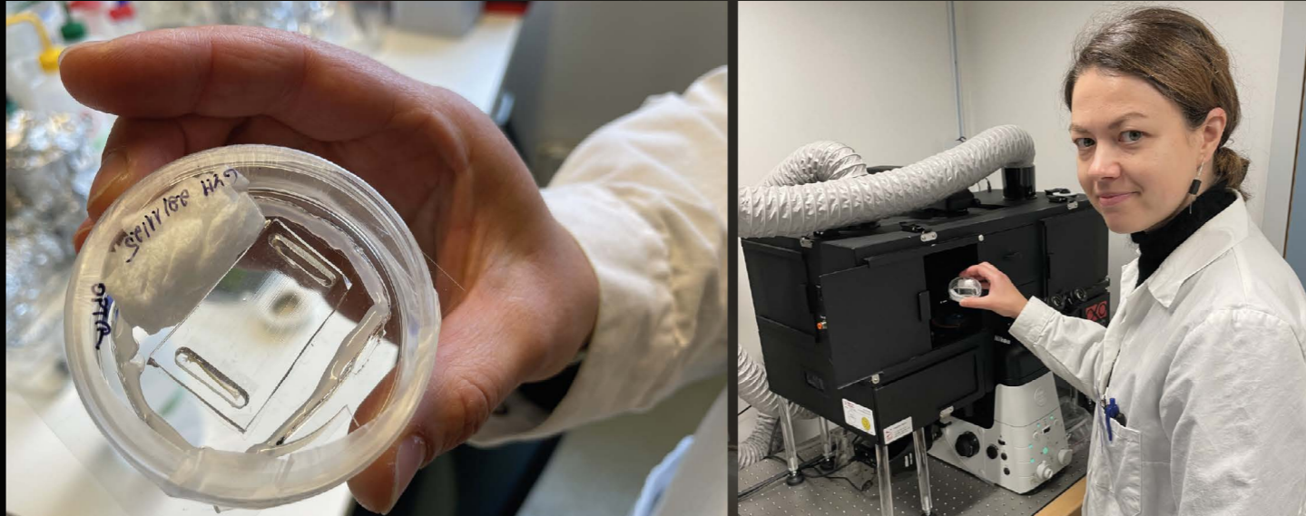
Photos were taken by Therese Ek. On the left, polydimethylsiloxane (PDMS) microstructured soil chip in a glass-bottom Petri dish is shown; on the right, Milda Pucetaite in the optical microscopy lab at Lund University.
